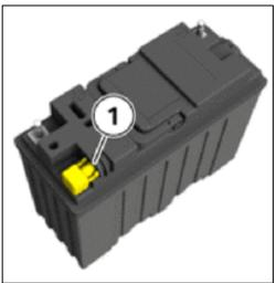
1 Install bleeding angular piece to the **NEW** No. 2 Battery.
